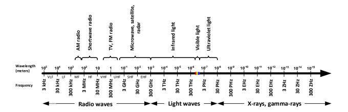
Unlike the visible light portion of the electromagnetic spectrum, RF can't be seen. Its presence and various characteristics such as frequency, wavelength, and amplitude can be detected and measured with specialized test equipment. Examples of that test equipment include signal level meters and spectrum analyzers.
