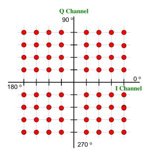
Figure 1: 64 QAM Constellation Display
